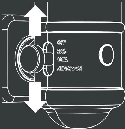
Flip the switch up or down to change the mode
